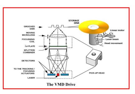
**Pick-Up Head:** Another vital component of the VMD player is the Optical Head (*pick-up*) that includes lasers, mobile actuators and lenses for picking up the reflected laser beam and passing it over to a multifaceted photodiode receptor which receives the signal from the VMD disc. VMD players require high quality optical *pick-ups*. Not all DVD *pick-ups* can be used for VMD player.
